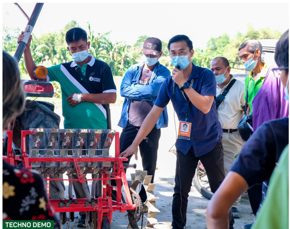
Engr. Marvin Estimada discussing the components of multi-row mechanical onion seeder
